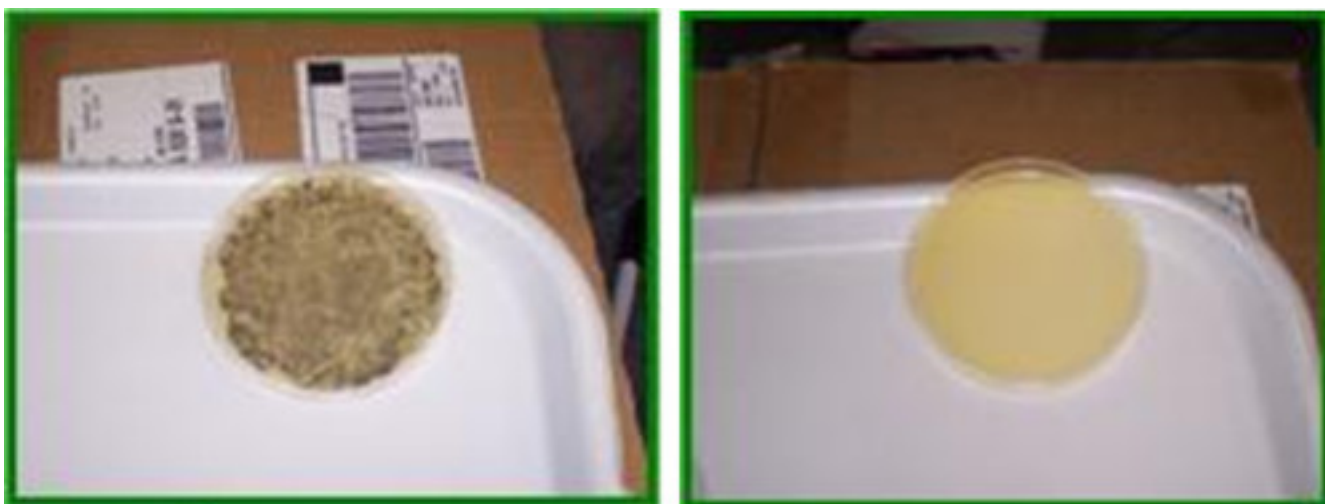
Figure 4. Visible growth of S. aureus colonies on untreated agar surfaces (left), and “no-growth” on agar surfaces treated with the D-FENS \text{ClO}_2 sprayer.
