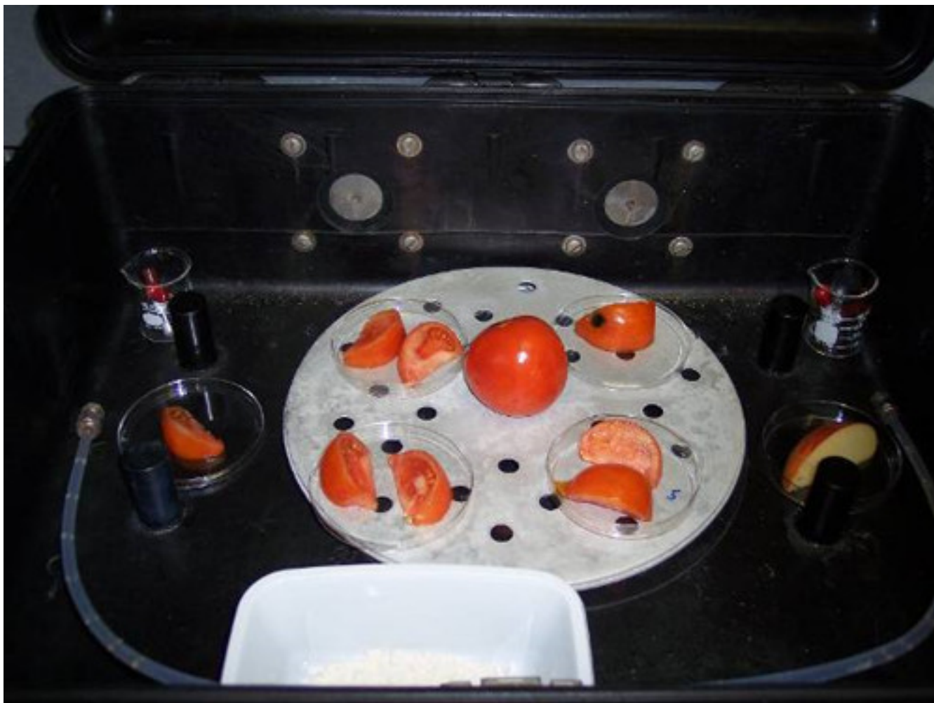
Figure 5. A typical PCS set-up to inactivate E. coli or L. monocytogenes on exterior tomato surfaces (center), browning enzymes in apple slices (right), and spore bio-indicators (back left and back right) 15 .
