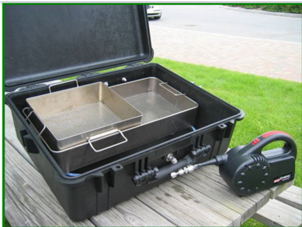
Figure 1. The PCS prototype derives from a rigid plastic PELICAN™ suitcase embellished with several design features to ensure sterilization while controlling pressure and temperature, and without off-gassing into the environment 15 .
