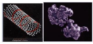
Tubular/fibrous: high aspect ratio particles
