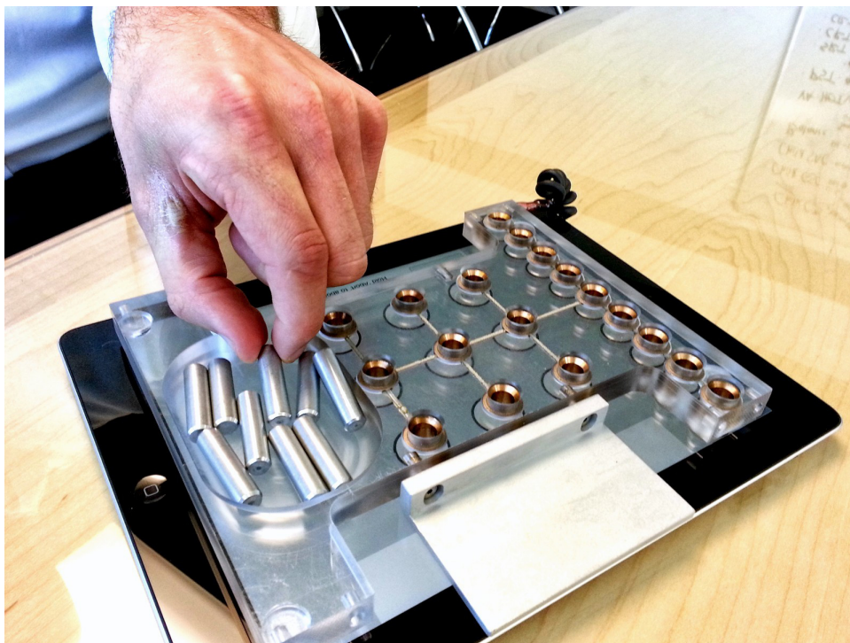
Figure 2. Manual dexterity test apparatus fitted to tablet.
