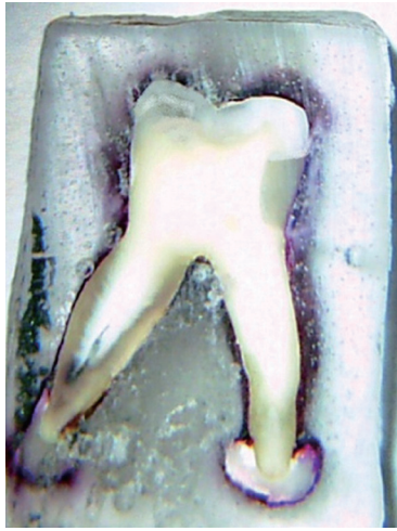
Fig. 4. A specimen with zero dye penetration after bonding the composite with Scotchbond Multi-Purpose.
