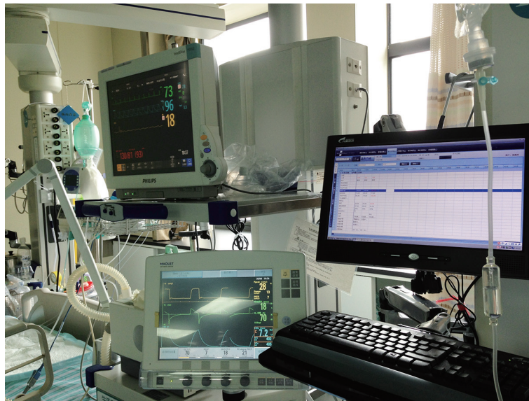
Figure 1 In Jinhua Municipal Central Hospital, every bed is equipped with a monitor (upper left) and a computer (upper right) so that data on vital signs (e.g., respiratory rate, heart rate, blood pressure and body temperature) and other physiological signals (e.g., extravascular lung water when transpulmonary thermodilution measurement is performed) can be automatically extracted from the monitor and stored in the electronic medical record (EMR) system in a predefined time interval. The lower screen displays parameters of ventilator setting, and these parameters can also be extracted to the EMR.
