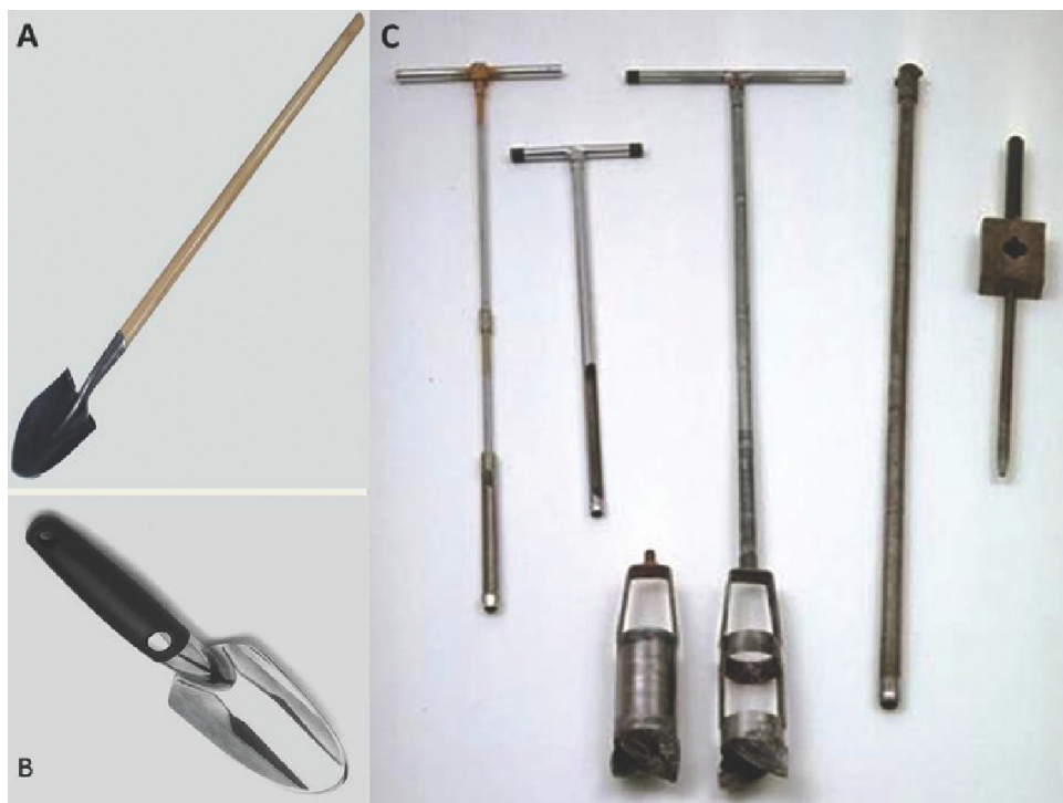
Figure 2. Shovels and other devices used for collecting soil samples. (A) Classic point-shovel. (B) hand shovel. (C) From left to right: Viehmeyer tube, trowel, oakfield tubes, soil corers.
