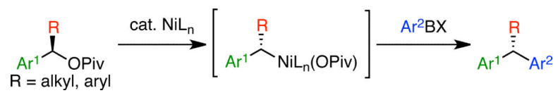
Scheme 1. Stereospecific Coupling of Benzylic Pivalates with Aryl Boroxines
