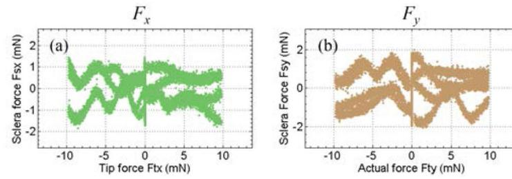
**Fig. 9.** Sclera force estimation error due to tool tip force. The calculated sclera force along X-axis  $F_{sx}$  versus the applied tool tip force along X-axis  $F_{tx}$  (a), and the calculated sclera force along Y-axis  $F_{sy}$  versus the applied tool tip force along Y-axis  $F_{ty}$  (b).
