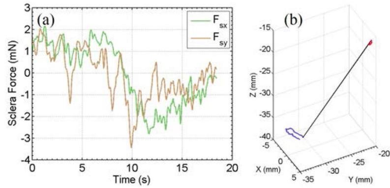
**Fig. 14.** Sclera force of one retina vein tracing trial (a). The corresponding trajectories of the sclerotomy point (red) and the tool tip (purple) (b). The black straight line shows the end position of the tool shaft.
