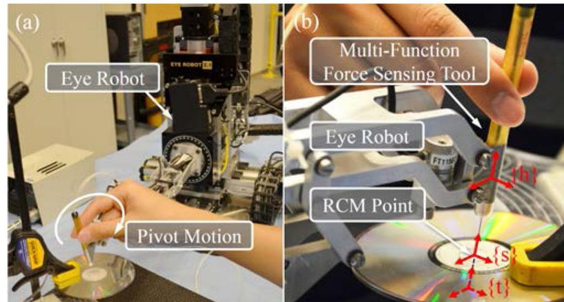
**Fig. 11.** Setup of the pseudo pivot calibration (a) and the close-up with coordinate frames robot handle {h}, sclera {s}, and tool tip {t} (b). Tool tip frame {t} is underneath the CD, shown with dashed arrows.
