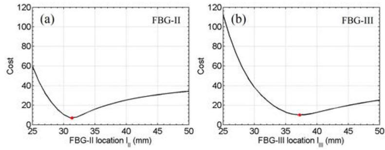
**Fig. 6.** Results of the optimization problem. The optimization cost for FBG-II versus  $l_{II}$  (a) and the optimization cost for FBG-III versus  $l_{III}$  (b). The red dots indicate the minimum cost where  $l_{II}^* = 31.3$  mm and  $l_{III}^* = 37.2$  mm.
