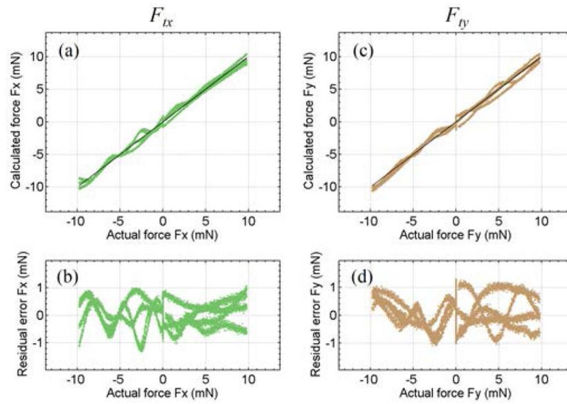
**Fig. 5.** Results of tool tip force calibration. The calculated tool tip force along X-axis  $F_{tx}$  versus the actual value (a), its residual error (b). The calculated tool tip force along Y-axis  $F_{ty}$  versus the actual value (c), and its residual error (d).
