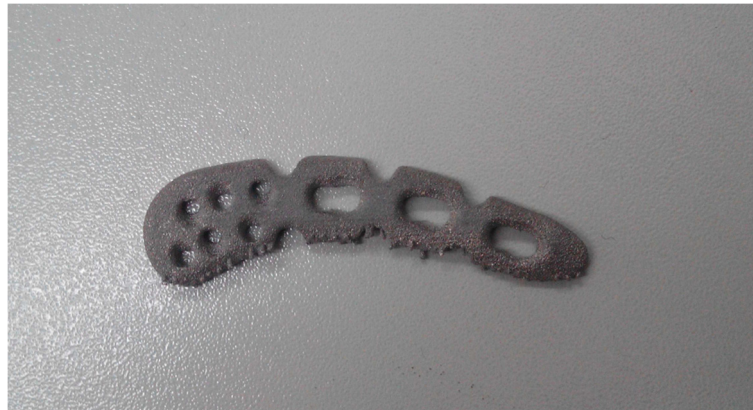
Figure 1 The EBM-printed Ti-6Al-4V LCP plate.
