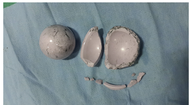
Fig. 3 – Fractured ceramic liner of acetabular component.
