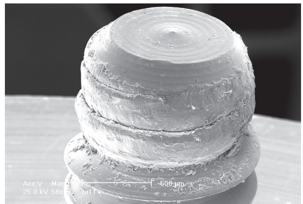
Figure 5- Scanning electron microscopy (SEM) micrograph demonstrating damages in the screw threads without fracture
