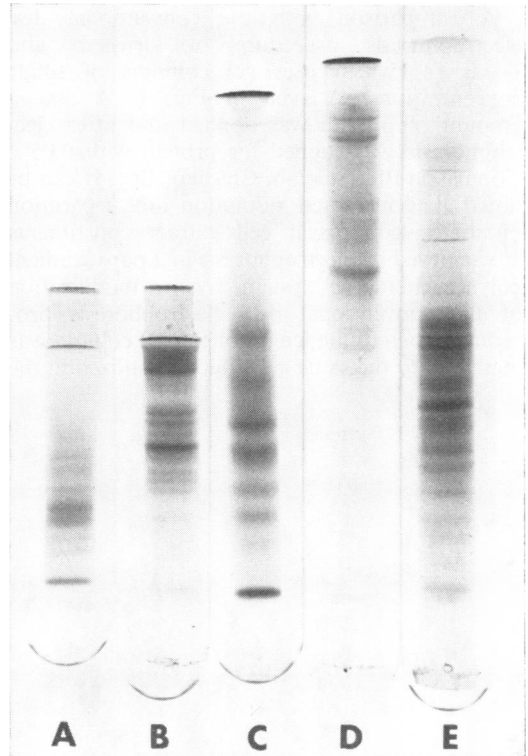
FIG. 1. Comparison of protein-stained profiles of M. tuberculosis culture filtrate samples as obtained by the conventional disc and the discontinuous pore gradient electrophoretic methods. Samples were subjected to electrophoresis in gel columns as follows (total gel concentration followed by gel height): A, 4.75% (6.5 cm); B, 7% (6.5 cm); C, 4.75% (8.5 cm); D, 7% (8.5 cm); E, four-stage discontinuous pore gradient polyacrylamide gel.
