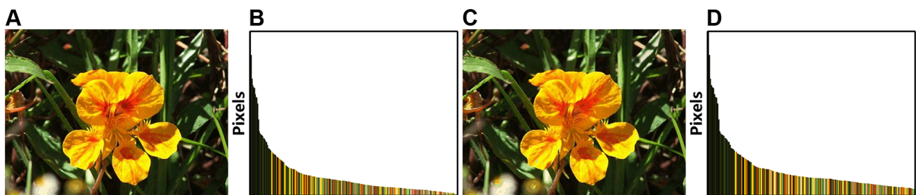
Figure 3. Replacement for low frequent colors with minimum variance quantization. (A) Minimum variance quantized Fig. 2A. (B) Color histogram of the image in A. (C) Full resolution output image resulting from the retained high frequent colors. (D) Color histogram of C. doi:10.1371/journal.pone.0112475.g003
