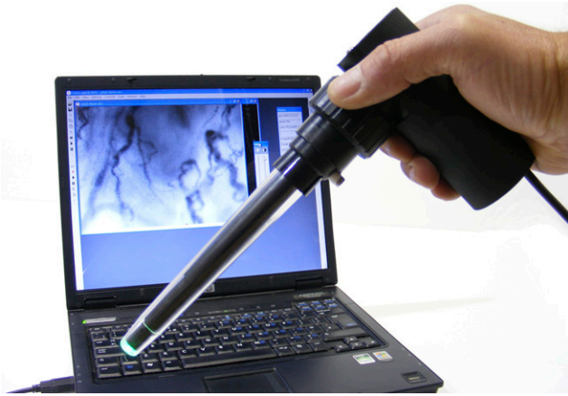
Figure 1. CapiScope handheld device connected to a laptop computer. Reprinted by permission from KK Technology.
