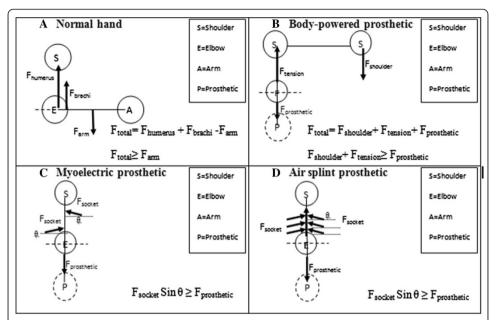
**Figure 2** Comparison of free body diagram from three different types of prostheses; **B.** Body-powered prosthetic, **C.** Myoelectric prosthetic, **D.** Air splint prosthetic and **A.** normal human hand. (S= shoulder, E= elbow, A= arm and P= prosthetic). The forces direction react referring to the x-axis and y-axis.
