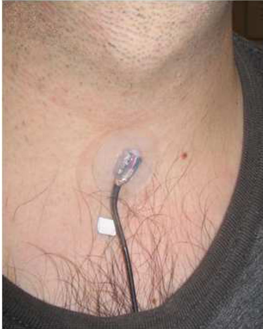
Fig. 5. (Color online) The accelerometer sensor mounted subglottally on the neck skin with double-sided tape.
