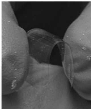
FIG. 1. Thin film of poly(propylene fumarate) (PPF) postcrosslinking. Thin films of PPF in various weight ratios with diethyl fumarate (DEF) were formed from 120 \mu L of polymer between 2×2 cm glass slides. Polymer crosslinking was initiated with 5 mg/g of bis(2,4,6-trimethylbenzoyl) phenylphosphine oxide (BAPO), under UVa light (3.5 mW/cm 2 ) for 90 min. Resulting thin films were 0.25 mm thick and weighed 0.15 g. The image shows a thin film composed of 2 g PPF to 1 g DEF (2:1).
