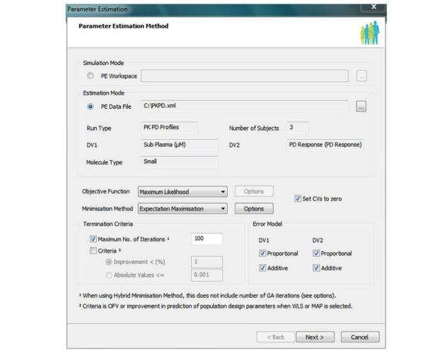
**Figure 4** A screen shot of the Parameter Estimation (PE) module that allows either of simulation or estimation modes. The observed clinical data are loaded in XML format and in the shown case the data include both plasma concentration and a PD response profile for simultaneous fitting of PK and PD dependent variables.
