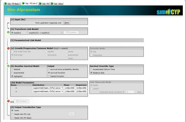
Figure 5 Simcyp screen representing a PD link response unit: input from the previous unit can go through a Link transform model and then feed into either a growth/progression/turnover model, survival model or custom scripted model.
