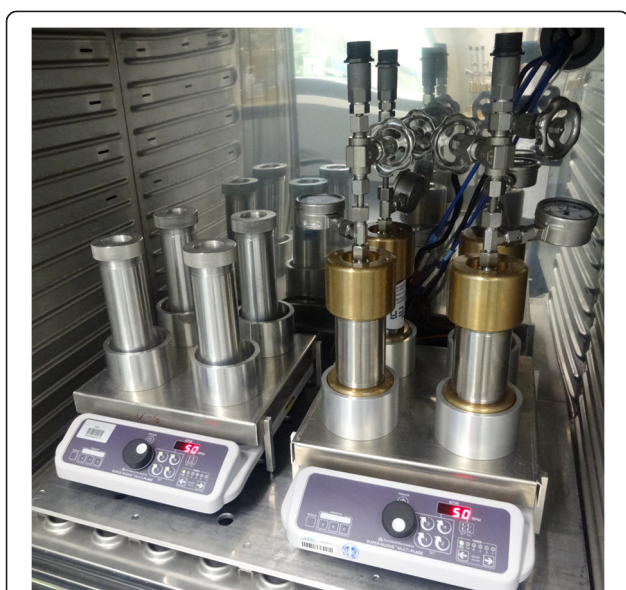
Figure 1 High-pressure reactors and control reactors. High-pressure reactors (right, made from stainless steel and bronze, max. pressure 40 MPa, pressurizing with N 2 gas, 160 mL volume) and aluminum control reactors (left, max. 0.1 MPa, 160 mL volume) were used for cultivation of hydrocarbon degraders at high and ambient pressure. The cultures were mixed with magnetic stirrers.
