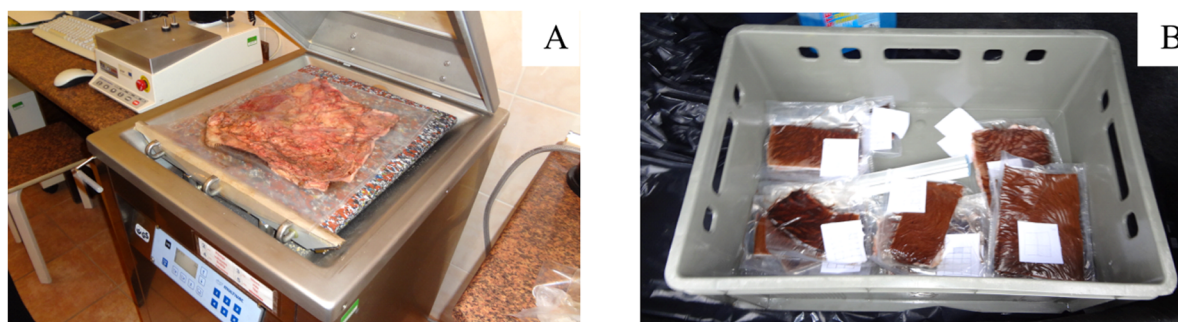
Figure 1. Equipment for fresh hide packing using vacuum (A) and the packed hide samples (B). doi:10.1371/journal.pone.0112783.g001
