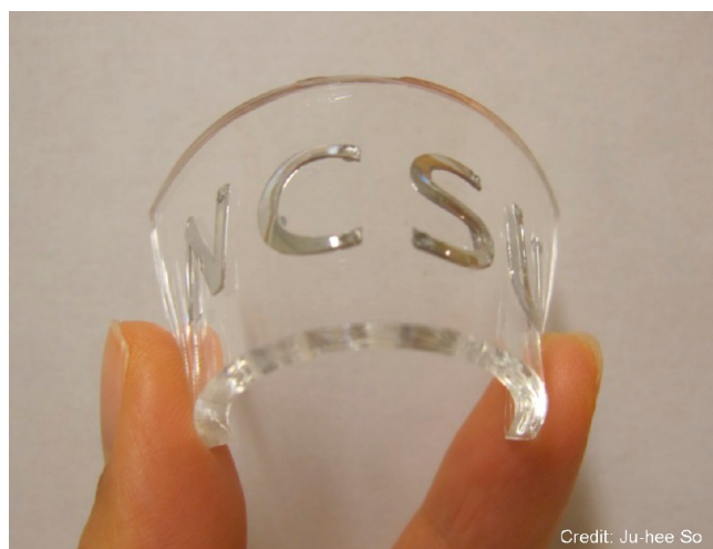
Figure 3. Microfluidic channels filled with EGaIn. The metal flows readily into microchannels by injecting it with a syringe, but stays in the microchannels in the absence of pressure because of the formation of the mechanically stabilizing surface oxide. The ability to deform the resulting metallic structures is limited only by the mechanical properties of the encasing polymer.
