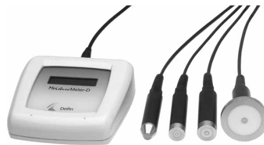
Figure 1 MoistureMeter-D with probes of four diameters. The probe used in this study was the third from the left, for an effective measurement depth of 1.5 mm.
