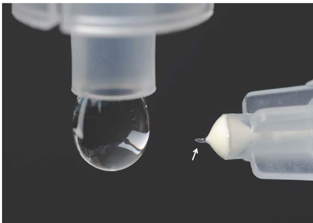
FIGURE 4. Hollow microneedle (arrow), 720 \mu\text{m} in length, is shown next to a liquid drop of approximately 50- \mu\text{L} volume from a conventional eye dropper.
