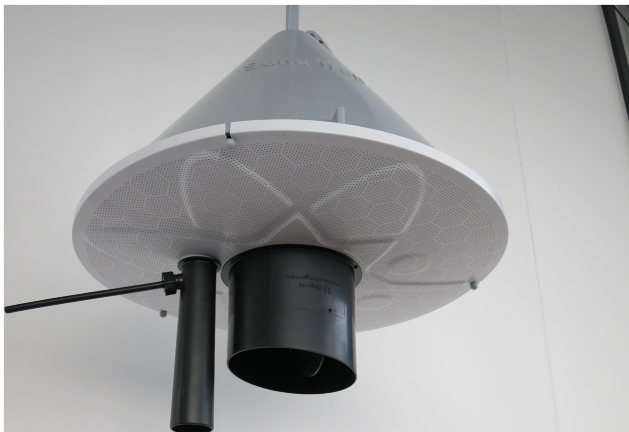
Figure 3 Suna trap with a plastic base with fine holes.
