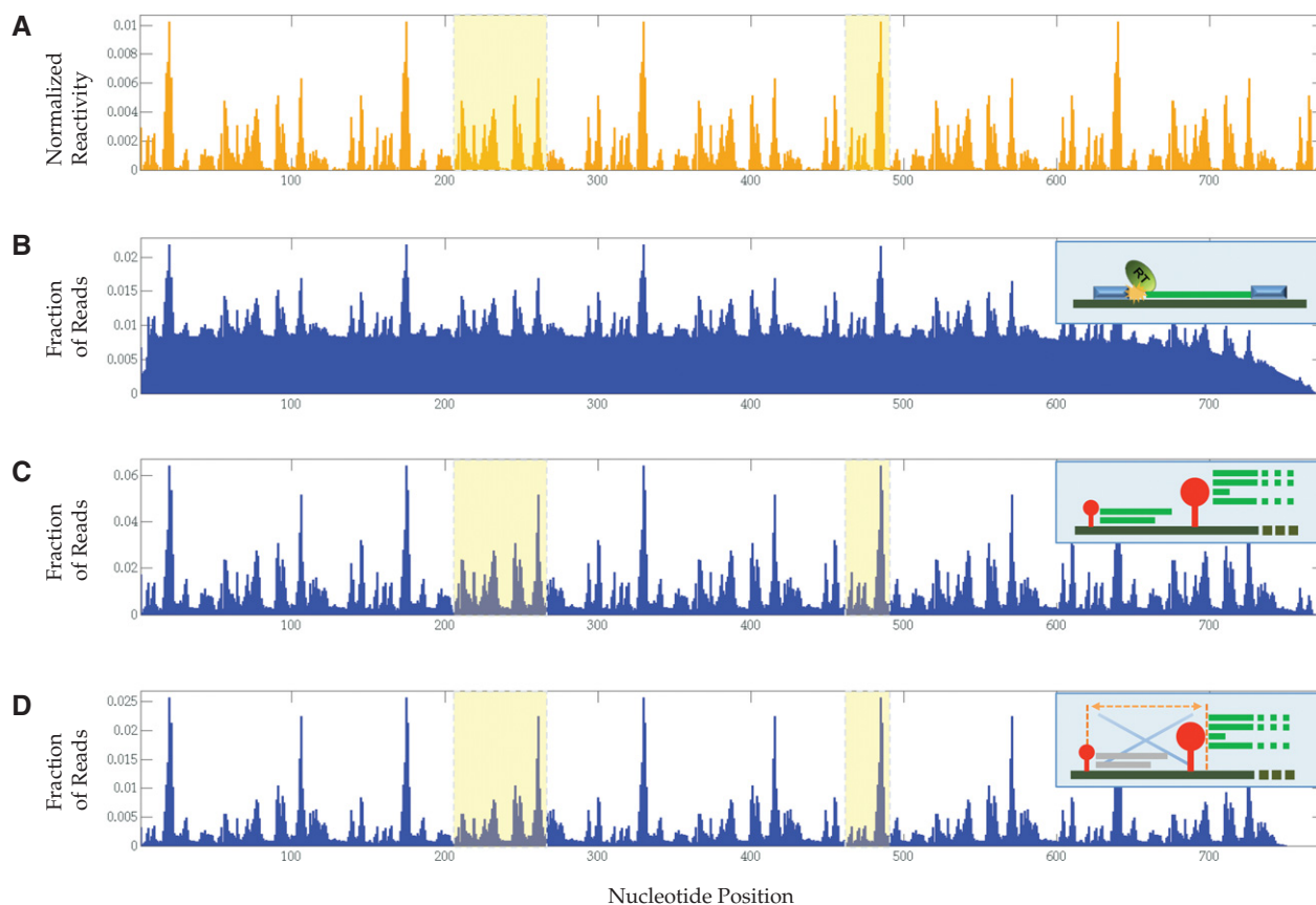
FIGURE 5. Read distribution in RPE experiment at different ratios of hit-to-primer rates and cDNA length ranges. (A) Normalized reactivity profile for a fictive RNA obtained by replicating the P546 SHAPE profile five times. Model-derived fractions of reads that reach each site at hit rates 0.003 (B) and 0.05 (C,D), with primer rate fixed at 0.01 and length range upper bounded at 500 nt. Signal decay intensifies when lower size cutoff of 25 nt is applied (D). Highlighted windows depict regions of signal decay.
