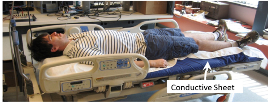
Fig 3. Human subject on conducting sheet that is connected to ground through monitoring circuit.
