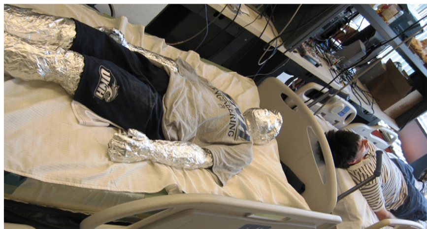
Fig 4. Measurement configuration with human subject and foil-covered dummy.
