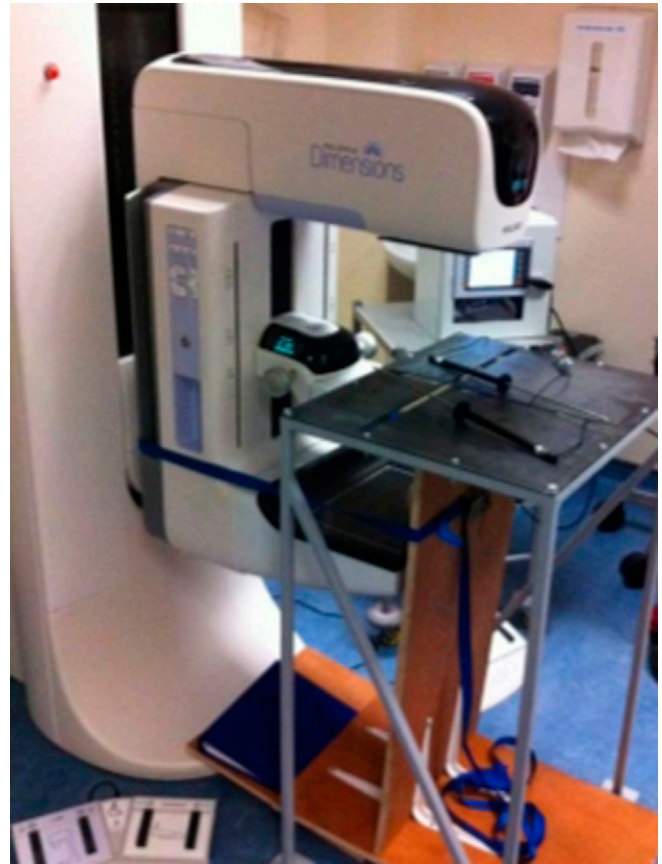
Figure 4. Deformable breast phantom mounted to rigid supporting board.
