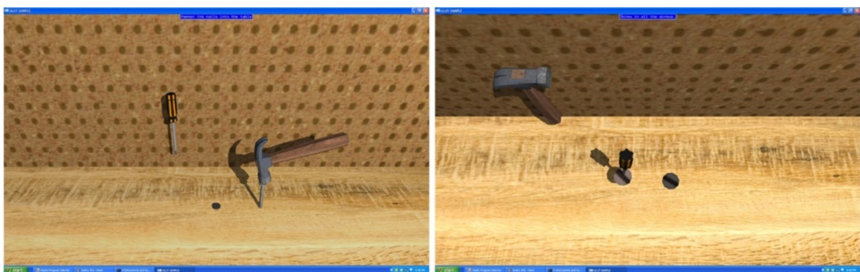
Figure 5 Tool use. The user needs to hammer the nails using the hammer and tighten the screws using the screwdriver. Left: hammering nails. Right: tightening screws. The hammer and screwdriver are grabbed by pressing a button the haptic stylus.
