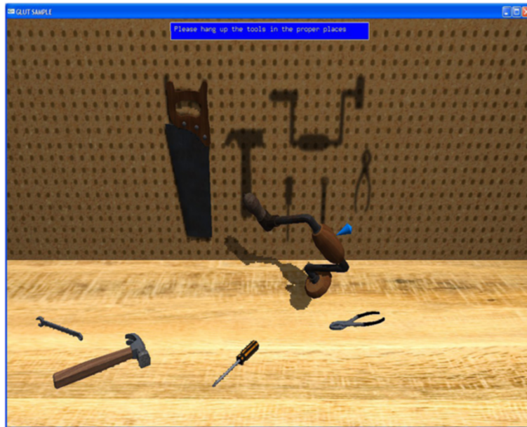
Figure 2 Workbench cleaning task. The user needs to pick tools and hang them on the backboard. The tools lock in place when their centroid is close to the center of the shadow.
