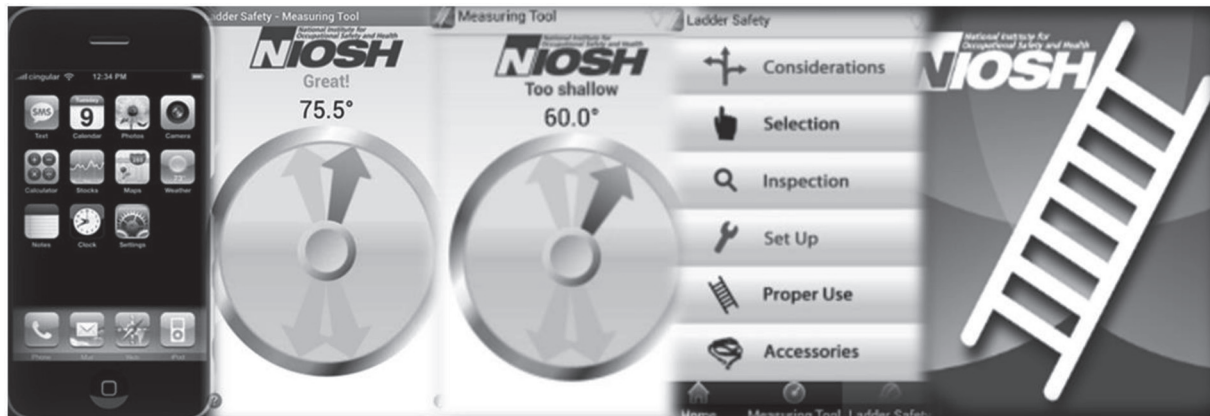
Fig. 3. A ladder safety software application (app) for mobile devices features a multimodal indicator and a graphic-oriented guide for ladder selection, inspection, positioning, accessorizing, and safe use (Simeonov et al. , 2013).
