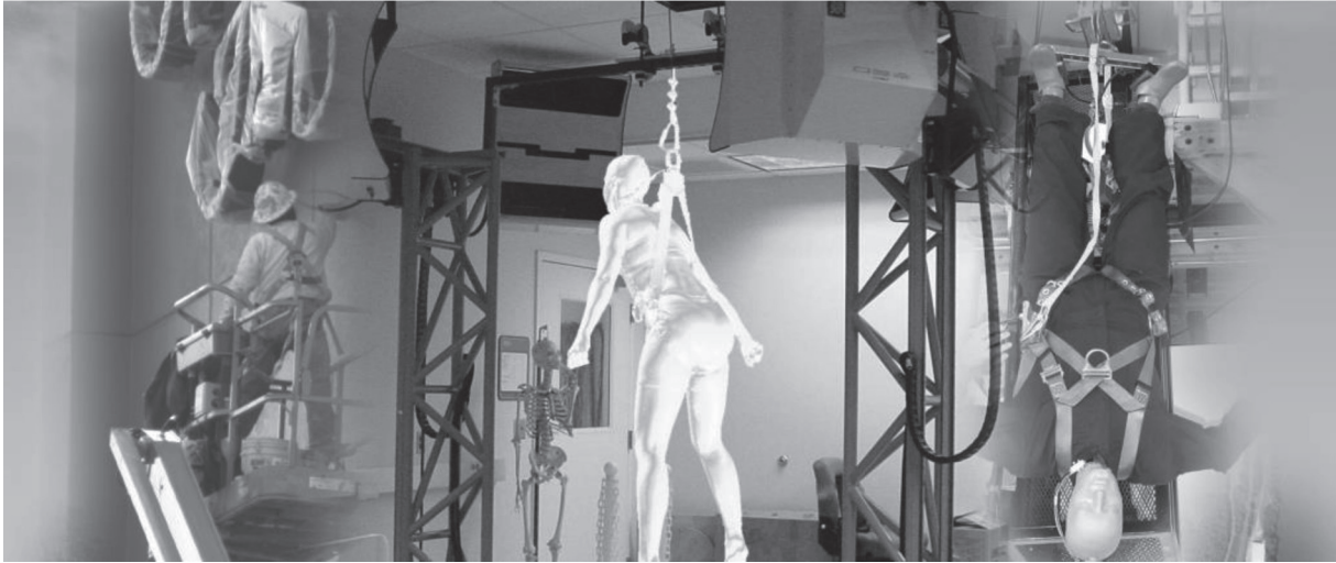
Fig. 5. NIOSH has had studies on harness sizing and design to accommodate diverse worker populations, suspension trauma risk, and how harness fit affects dynamic loading to the head and neck during fall arrests.
