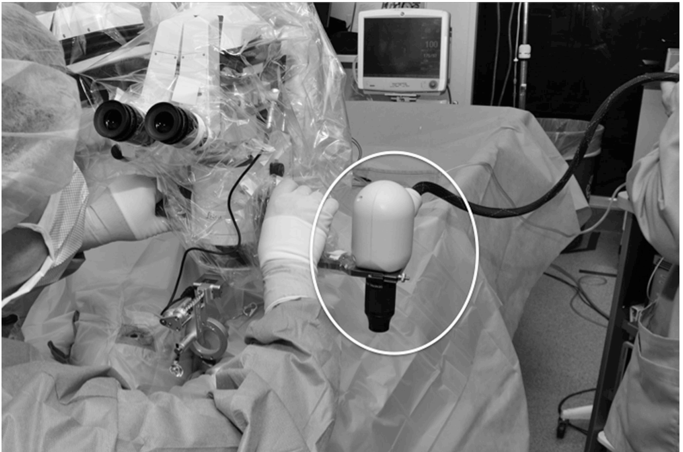
Figure 1. Microscope-mounted portable spectral domain optical coherence tomography system (circle).
