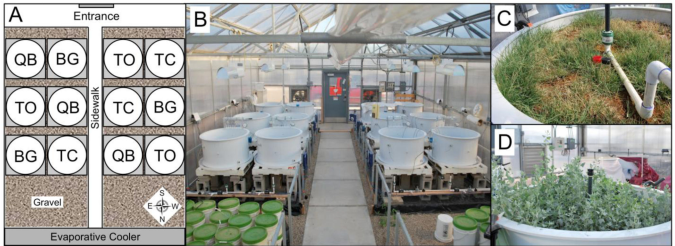
Figure 1. Greenhouse mesocosm experiment. (A) Schematic diagram showing the spatially randomized arrangement of the mesocosm treatments at the greenhouse ( TO , tailings only; TC , tailings + 15% w/w compost; BG , tailings + 15% w/w compost + buffalo grass; QB , tailings + 15% w/w compost + quail bush). (B) Picture of mesocosm containers prior to the start of the experiment. (C) Buffalo grass plants at t_3 . (D) Quail bush plants at t_3 .
