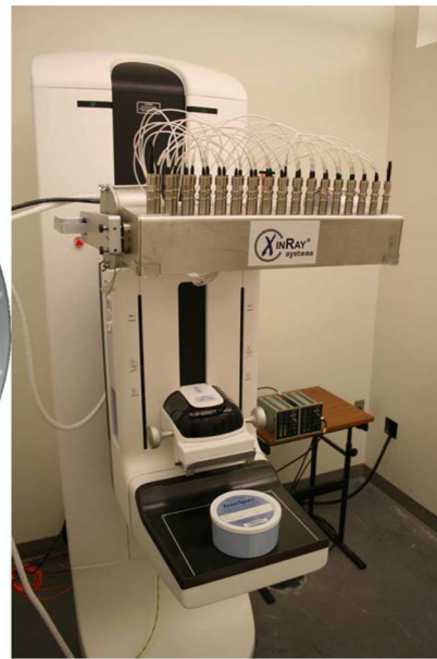
Figure 1. Left - - Segmented 2D radiograph of container used to hold specimens. Right - Image of an s-DBT system with specimen container on the detector housing.
