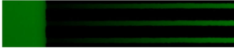
Figure 10.4. Spatial gradient of fluorescence along the cell migration channels. The cell loading chamber on the left also shows up in fluorescence because of the order of magnitude increased thickness.
