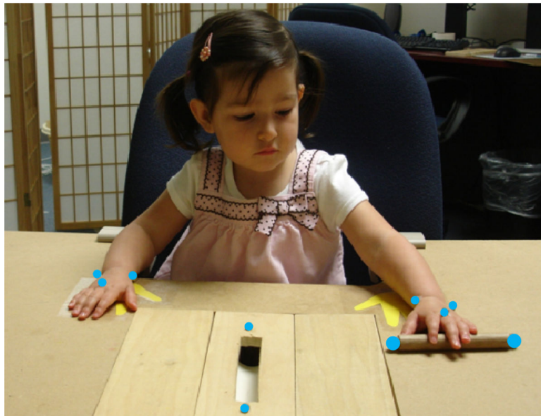
Figure 1. The experimental setup – depicted here is a horizontal rod and vertical slot presented on the left hand side. Markers were placed on the 3 rd metacarpal (knuckle), ulnar styloid (wrist), radial styloid (wrist), ends of the rod, and ends of the slot.
