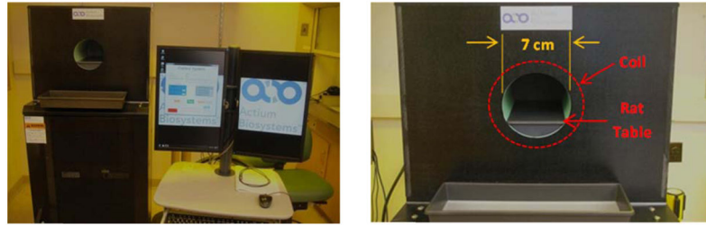
Figure 1. Induction coil chamber and power supply of a small animal magnetic field hyperthermia system (Actium Biosystems) with thermal monitoring and control console.
