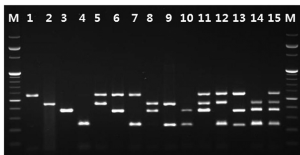
Fig. 4. Simultaneous detection of all possible combinations among SPCFV, SPVC, SPV2, and SPSMV-1 by multiplex RT-PCR. Lane M: 100 bp ladder; Lane 1: SPCFV; Lane 2: SPVC; Lane 3: SPV2; Lane 4: SPSMV-1; Lane 5: SPCFV and SPVC; Lane 6: SPCFV and SPV2; Lane 7: SPCFV and SPSMV-1; Lane 8: SPVC and SPV2; Lane 9: SPVC and SPSMV-1; Lane 10: SPV2 and SPSMV-1; Lane 11: SPCFV, SPVC, and SPV2; Lane 12: SPCFV, SPVC, and SPSMV-1; Lane 13: SPCFV, SPV2, and SPSMV-1; Lane 14: SPVC, SPV2, and SPSMV-1; Lane 15: SPCFV, SPVC, SPV2, and SPSMV-1.
