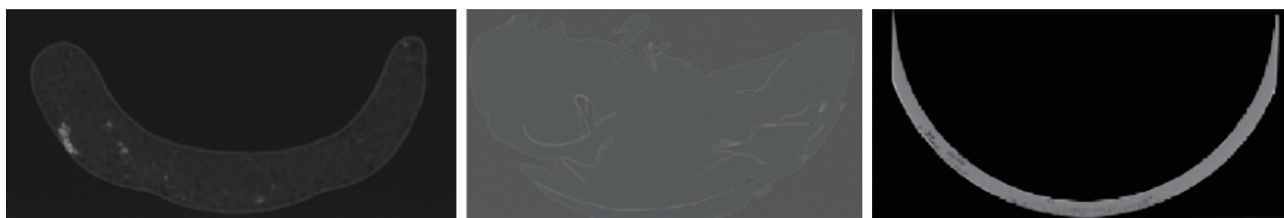
Figure 7 CT images of immobilization devices whose heterogeneity and lack of part-to-part reproducibility makes them unsuitable for proton therapy immobilization
