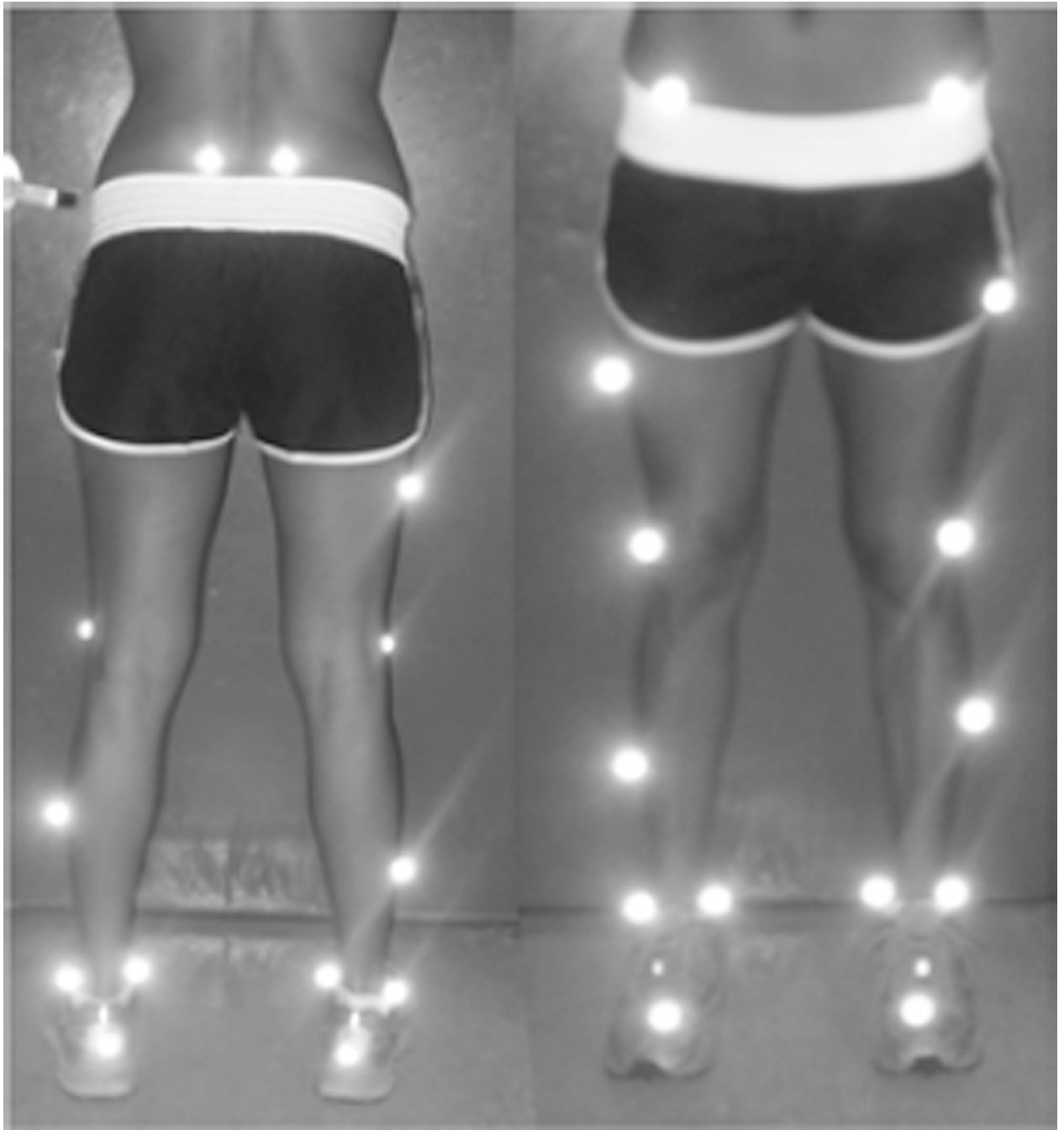
Figure 1. Plug-in-gait Model Retro-reflective Marker Setting (Vicon Motion System, Denver, CO).
