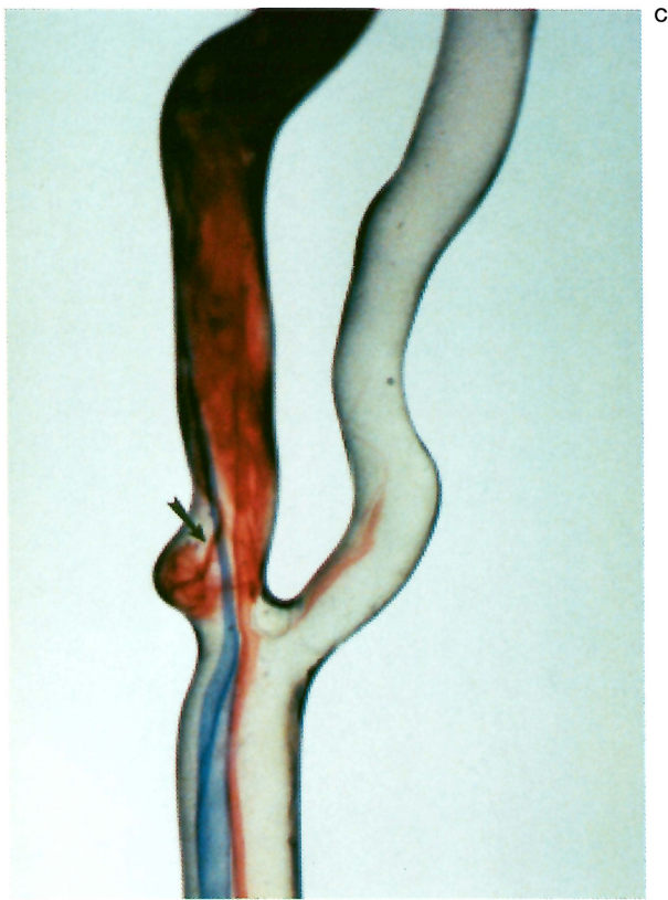
Figure 2 Ulcer entry and exit flow analysis. A) There is slipstream entry into the distal neck of the ulceration (arrow). B) Sluggish swirling slipstreams in a reverse vortex pattern are seen within the ulceration. C) Injections into different slipstreams show an opacified slipstream exiting the proximal neck of the ulcer (arrow) and being sucked into the central jet of the stenosis.
