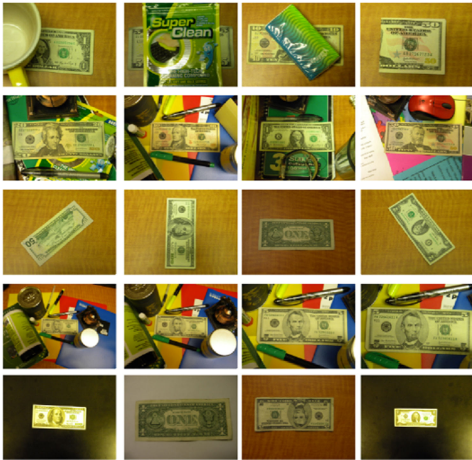
Figure 5. Samples of banknote images taken under different conditions: 1 st row (partial occlusion), 2 nd row (cluttered background), 3 rd row (rotation), 4 th row (scaling change), and 5 th row (illumination change).
