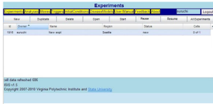
Fig. 3. Start, Pause and Resume buttons of DISimS to allow pausing an ongoing simulation and resuming with a different set of input parameters in a single experimental simulation run
