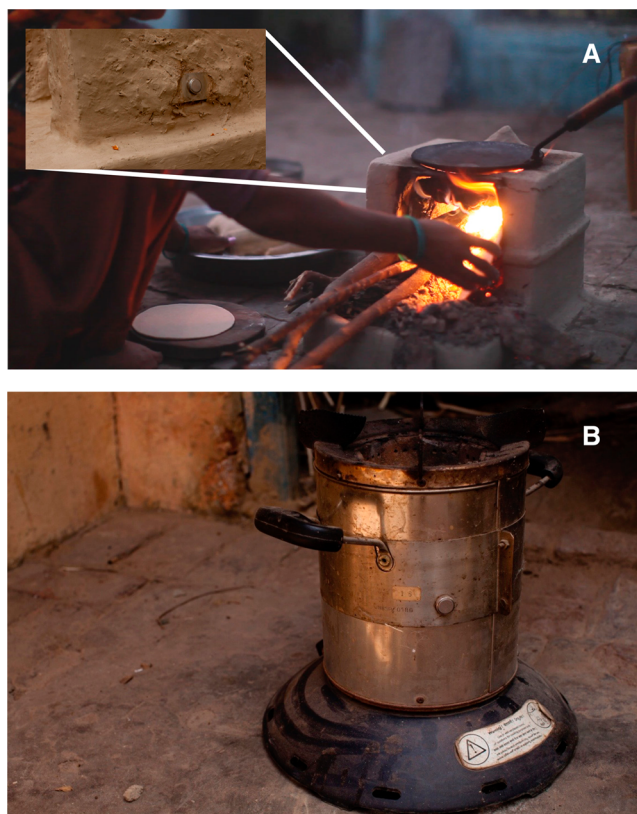
Figure 1. Traditional and intervention stoves and placement of stove use monitors. (A) Typical traditional wood and dung-fueled stove. The inset image shows the Stove Use Monitor and its holder. (B) The Philips intervention stove. A metal sheet stamped with a unique identifier and machined with a hole was used to securely hold each stove use monitor.
