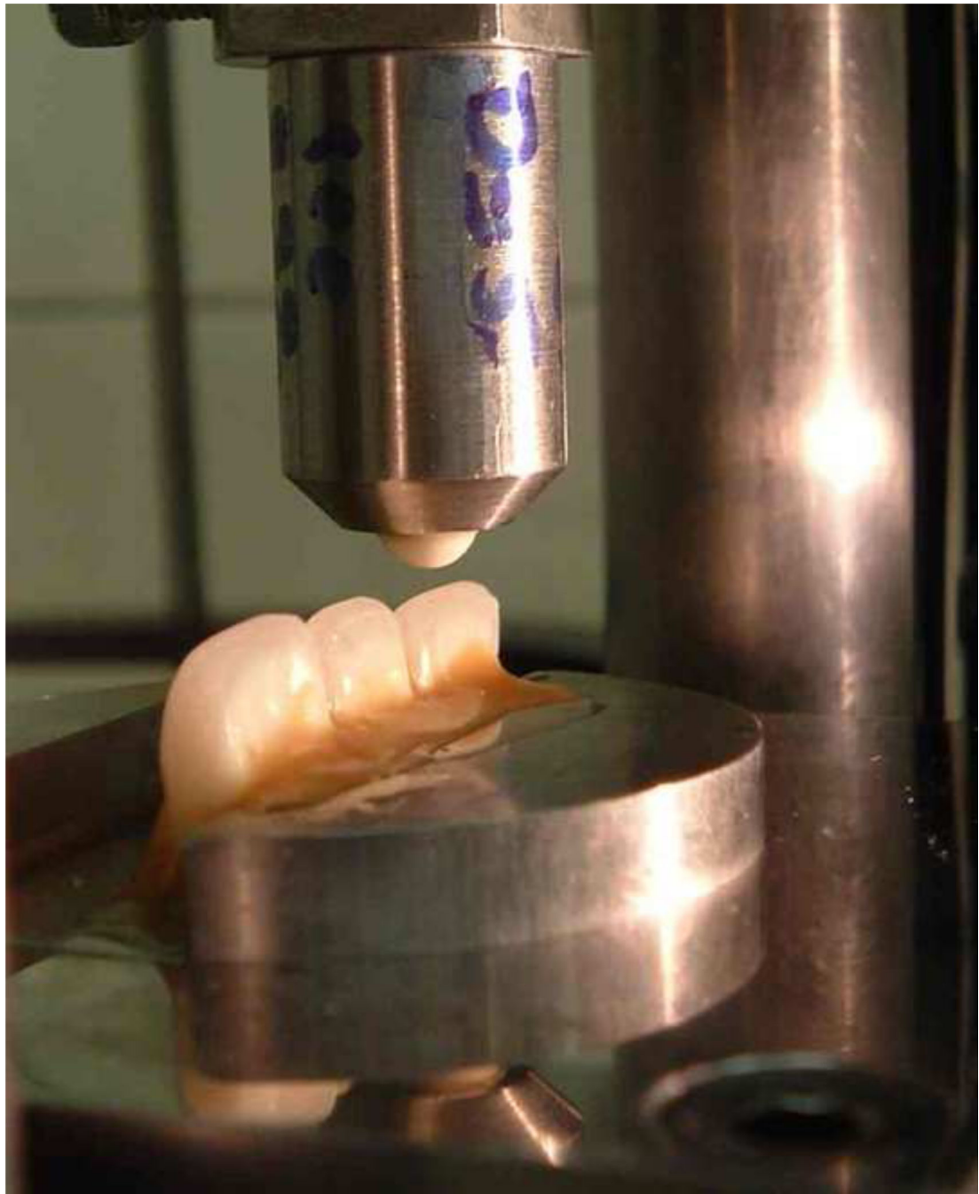
Fig. 2. Edge chipping may be done on simple bocks or actual teeth as shown here. (a) and (b) show a sharp 120^\circ conical indenter indenting into three teeth mounted side by side. Flats have been ground into the incisal and lingual faces to make a 90^\circ edge. (c) shows a 5 mm alumina ball indenter about to indent three teeth with no flats.
