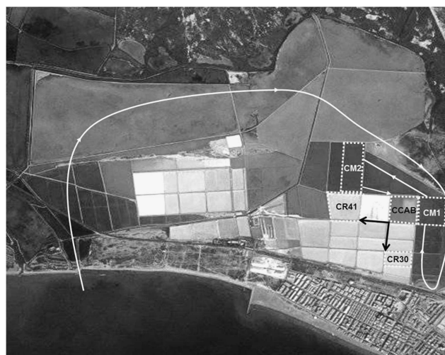
Figure 1 Aerial photograph of Bras del Port saltern ponds, Santa Pola, Alicante. Water is pumped from the sea to preconcentrators, medium concentrators, a brine concentrator and finally to the crystallizers. The ponds analyzed in this study are framed with dotted white lines: CM1 and CM2 (medium concentrators), CCAB (brine concentrator) and CR30 and CR41 (crystallizers). Arrows indicate the water circuit.
