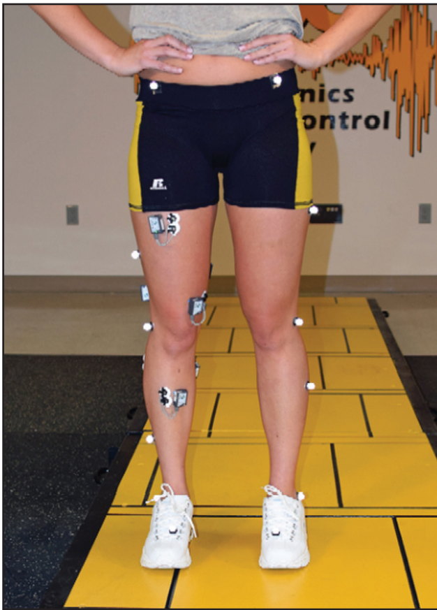
Figure 1. Placement of reflective markers. A leg warmer was used on the right leg to help stabilize the EMG electrodes.
