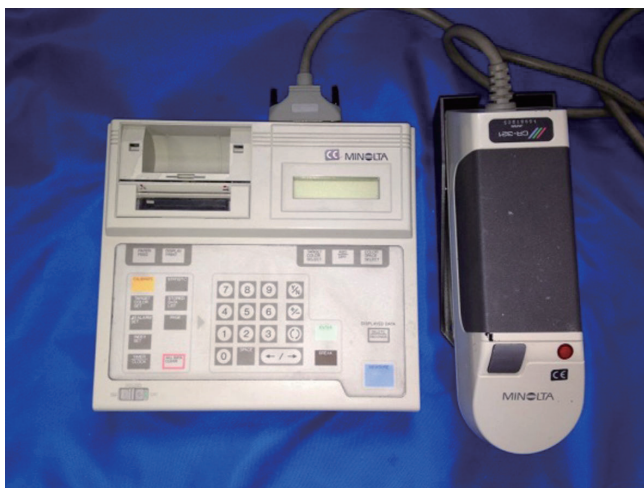
Fig. 2. Colorimeter (Minolta CR 321; Konica Minolta, Tokyo, Japan).
