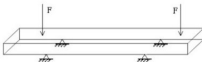
Figure 8. Schematic diagram of concrete bridge FEM model.
