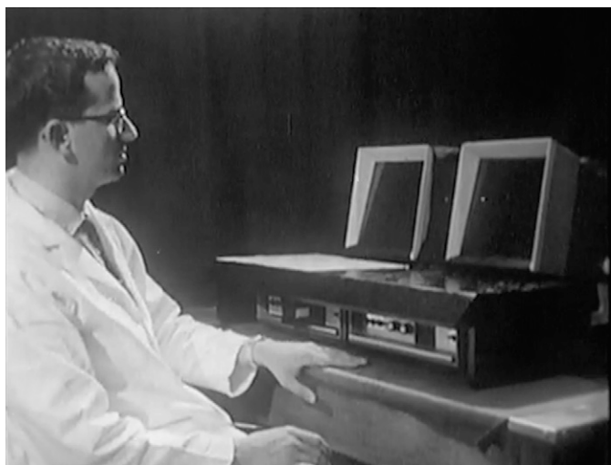
The author displays one of the tachistoscopes he built for the first tests of split-brain subjects.
