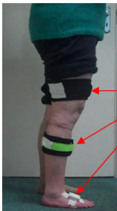
Figure 1 Inertial sensors secured to thigh, shin and foot.
