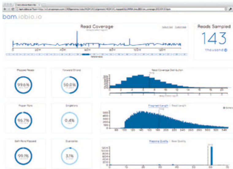
Figure 1. The bam.iobio.io web application. The user selects an alignment file, and the application rapidly samples the entire file to estimate genome-wide averages for a set of informative alignment metrics. Additionally, the user is able to select specific regions of interest and redo the analysis in those regions in seconds.
